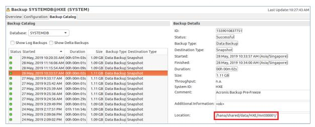
During a recovery, we will first recover the folder containing a snapshot, and then revert the databases to this snapshot by using SAP HANA Studio.
